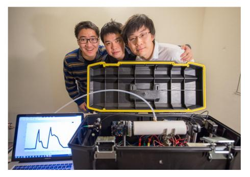
So, this is the first product we built. It mainly servers the oil and gas industry. Traditionally if you want to inspect gas pipelines or gas stations or any leaks, this device will help you identify them.
